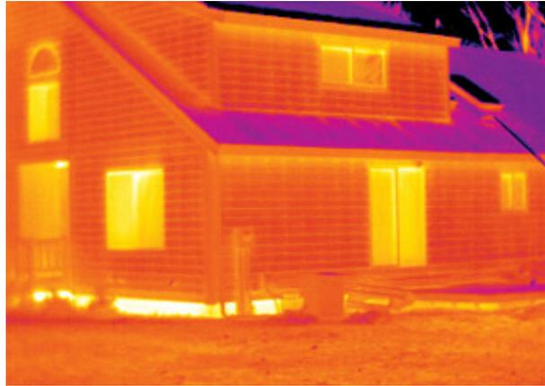
Thermal Infrared image of a house, clearly showing radiation passing through glass windows.
